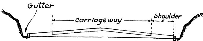
Cross section of road carried in cutting. The formation width is the total width between side gutters.
