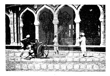
Fig. 49.—Barrel Pump in action. (Author's?original photo).
