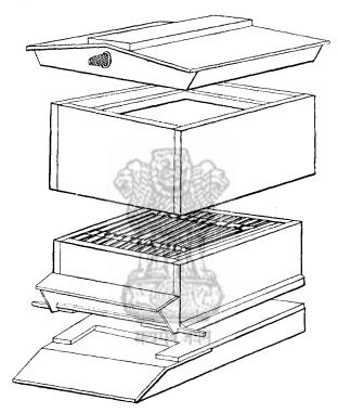
Fig. 95.—Diagrammatic sketch of a Bar-frame Bechive, showing construction.
